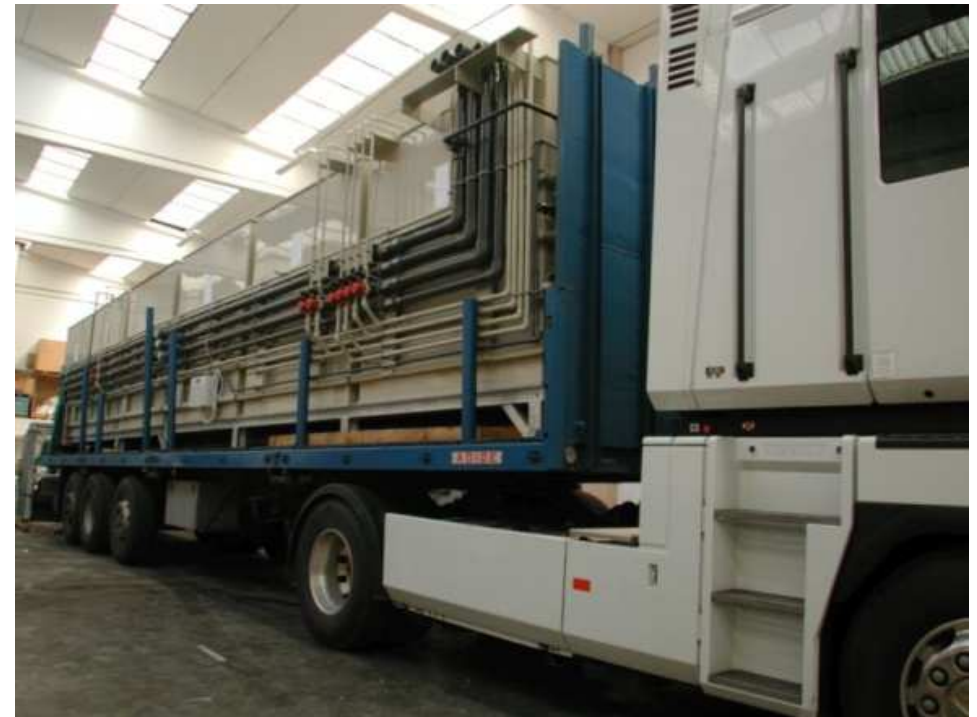
Section of reaction tanks, loaded on truck and ready for shipment 16
